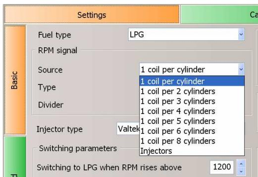
\* The type of signal - signal sensitivity, threshold voltage above which will read the signal turns. Value to choose from depending on the location from where is the speed signal.
