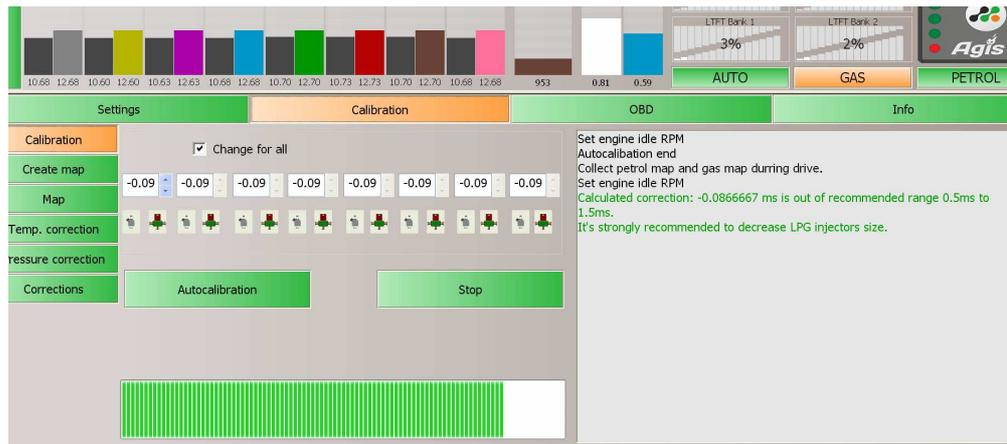
After the selection: speed signal, switching parameters, temperature sensors / if used other than the supplied / , gas level sensor, a gas injector, we can begin the process of auto-calibration for this purpose, press the button and leave AUTOCALIBRATION car idling.
